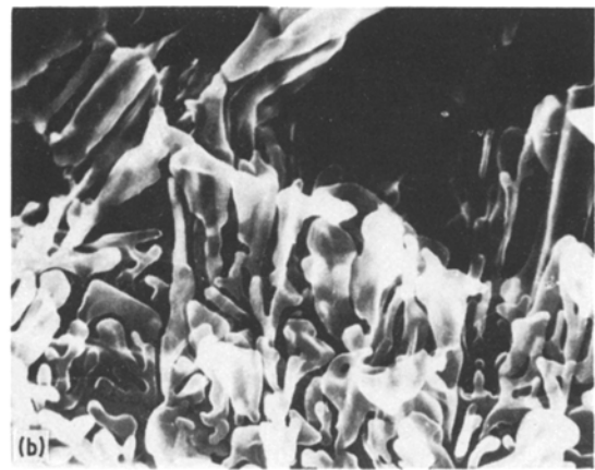
Figure 4 (a) The initial silicon crystals and (b) the silicon eutectic crystals on the surface of the carbon fibres etched from the matrix, (a) \times 1350 , (b) \times 4500 .
